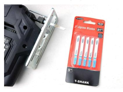
It's best to use a jigsaw with metal blades – (21 TPI). Go very slowly and steadily otherwise you risk breaking the blade or causing enough heat as to melt the polycarbonate...and getting the blade stuck to the box.
