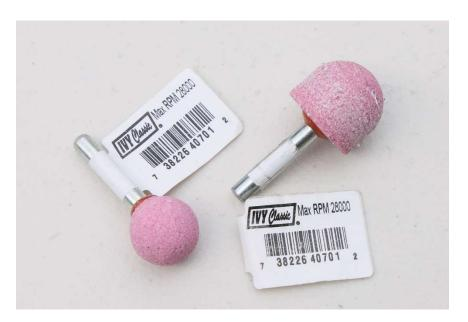
These above, or similar, can be used in a drill to soften the edges of where you sawed. You can alternately use gaffing tape to cover the edges as they are all between the netcam and the back post and would not be near players.
