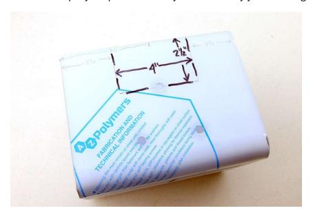
Mark off a section of approximately  $4" \times 2-1/2"$  either on a new unit, or by using a Sharpee<sup>TM</sup> on an existing unit. This will need to be removed so that the netcam can sit a bit further back on the platform. The limit of your placement would then be the top of the camera.
